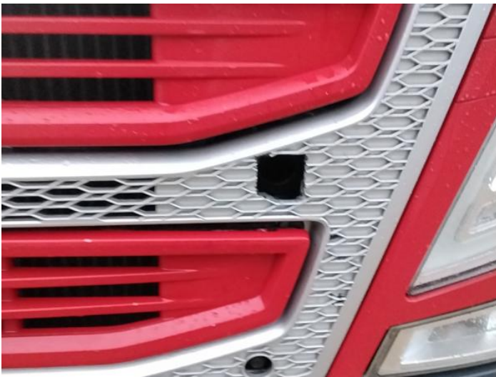
5: Front TowEye Cvr Missing Replace
