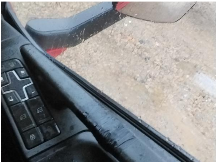
15: Handle Inner osf Damaged Replace
