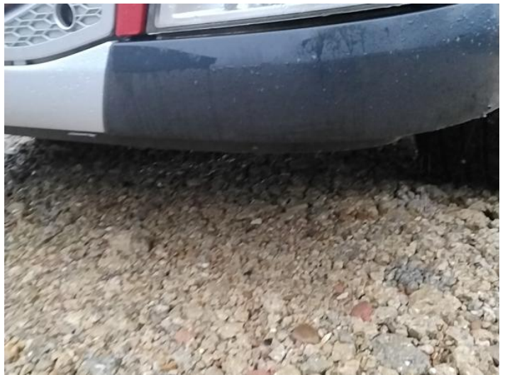
6: Bumper Front Moulding Missing Replace
