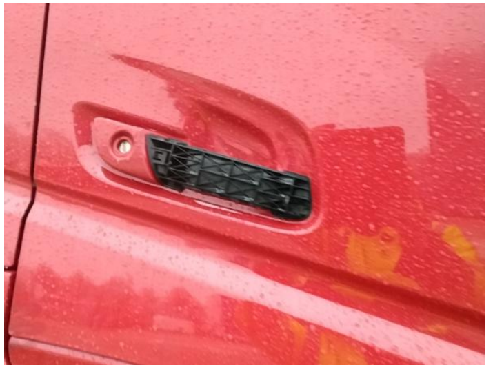
12: Handle Outer osf Missing Replace
