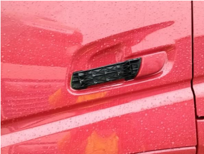
9: Handle Outer nsf Broken Replace
